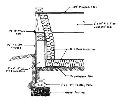
Underfloor Return Air Plenum With Pressure Treated Wood Foundation
